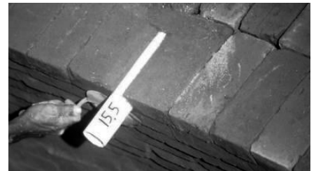
Fig. 9. Resonator for 622 Hz.
