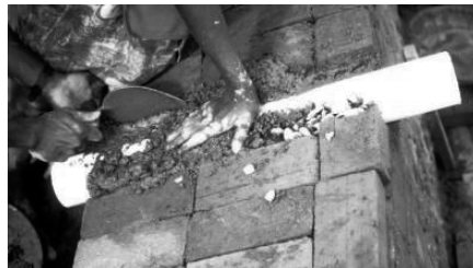
Fig. 8. Resonator for 219 Hz.
