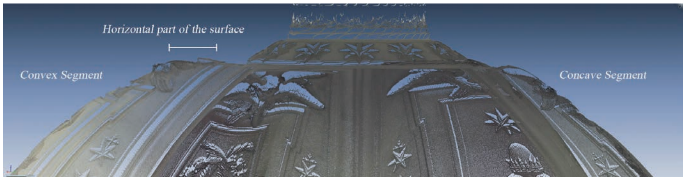
Fig. 18. Section in Convex segment of the Dome's point cloud shows the horizontal part at the top covered by the decorative angel.
