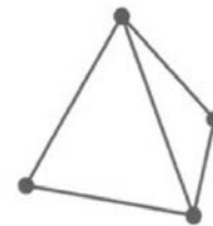
Fig. 14. Four-sided element with line function shape used for calculation (Zamani, 2011, [11]).
