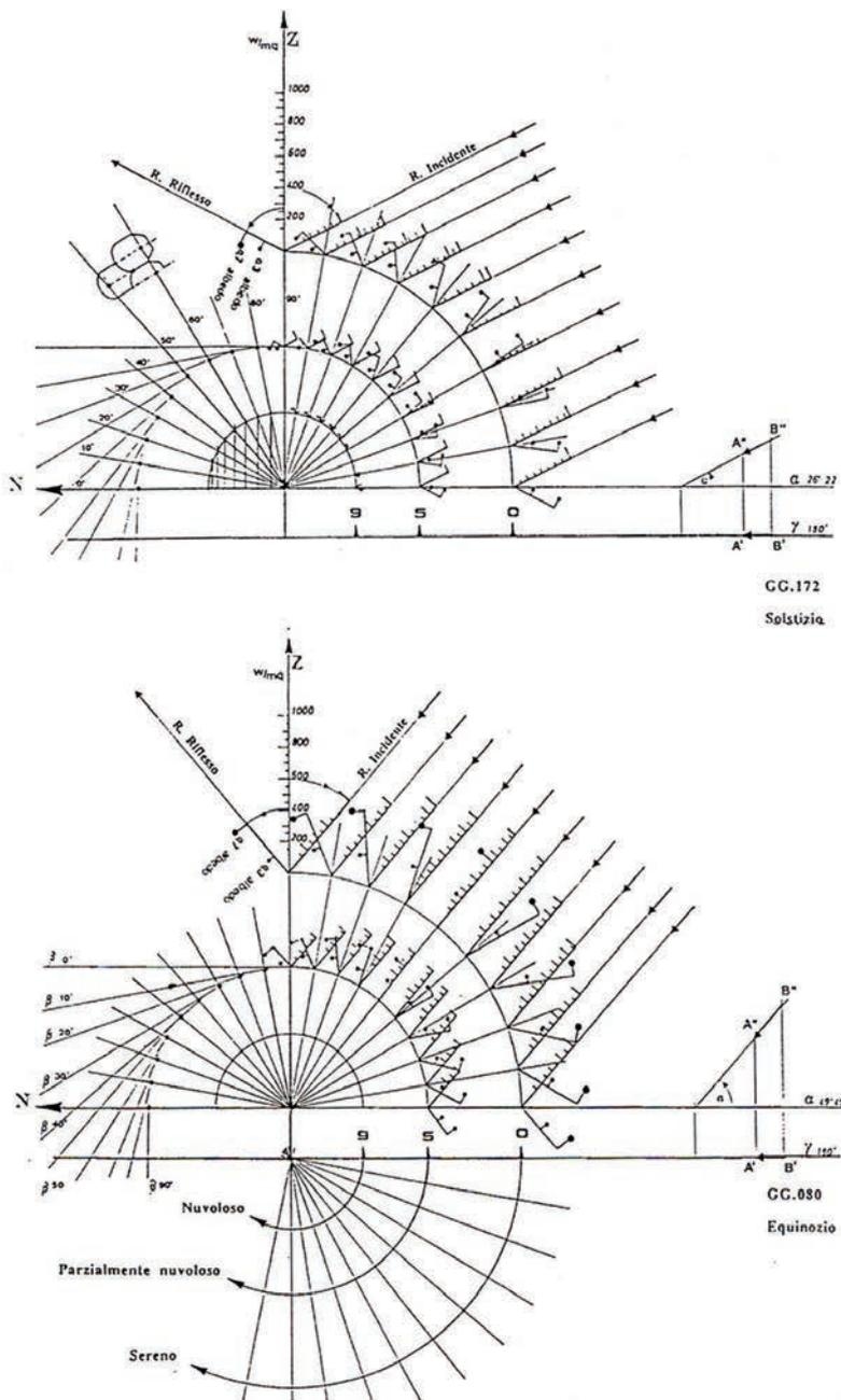
Fig. 6. Diagram of the incident and reflected radiation for surfaces. The balance is obtained for green glazed terracotta tiles ( $a = 07$ , internal dot) and yellow glazed terracotta tiles ( $a = 039$  external dot) inclined every 10 degrees with respect to the dome shell and calculated at the latitude of Naples for the spring equinox and the summer solstice at 7 am and 1 pm in sunny (0), partially cloudy (5) and cloudy (9) conditions (data obtained from the meteorology station of Capodichino)
