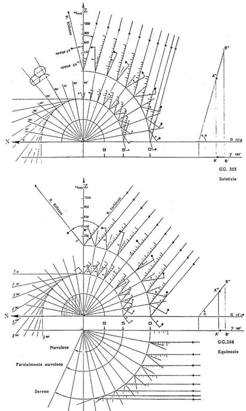
Fig. 5. Diagram of the incident and reflected radiation for surfaces. The balance is obtained for green glazed terracotta tiles ( $a = 07$ , internal dot) and yellow glazed terracotta tiles ( $a = 039$  external dot) inclined every 10 degrees with respect to the dome shell and calculated at the latitude of Naples for the spring equinox and the summer solstice at 7 am and 1 pm in sunny (0), partially cloudy (5) and cloudy (9) conditions (data obtained from the meteorology station of Capodichino).
